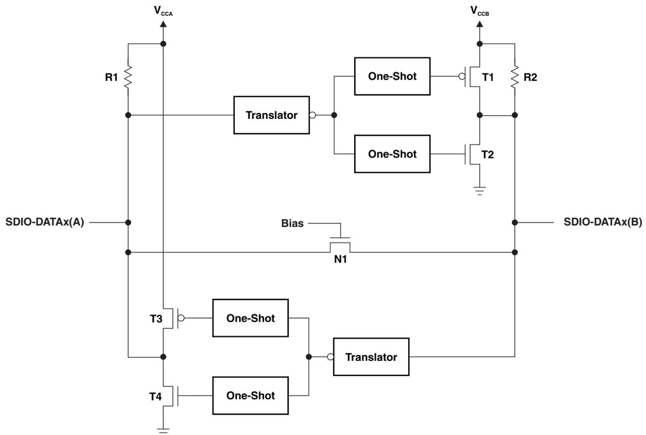
Figure 27. Architecture of an SDIO Switch-Type Cell
