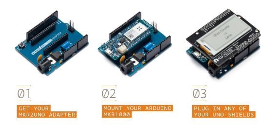
Like in many others Arduino boards this adapter allows to power your MKR board using a barrel jack with center positive polarity or the VIN pin on the headers.
