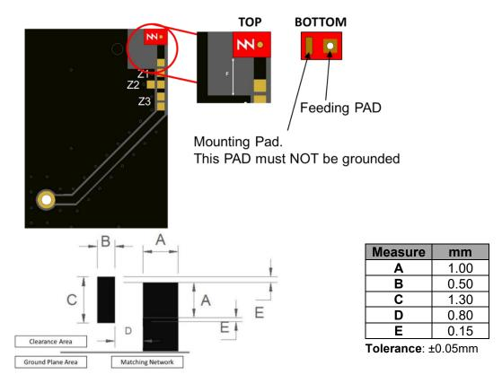
Footprint dimensions for the NANO mXTEND™ (NN02-101) antenna booster (in the corner).
