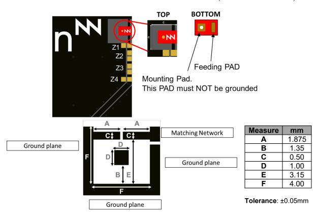
Footprint dimensions for the NANO mXTEND™ (NN02-101) antenna booster (in the middle).
