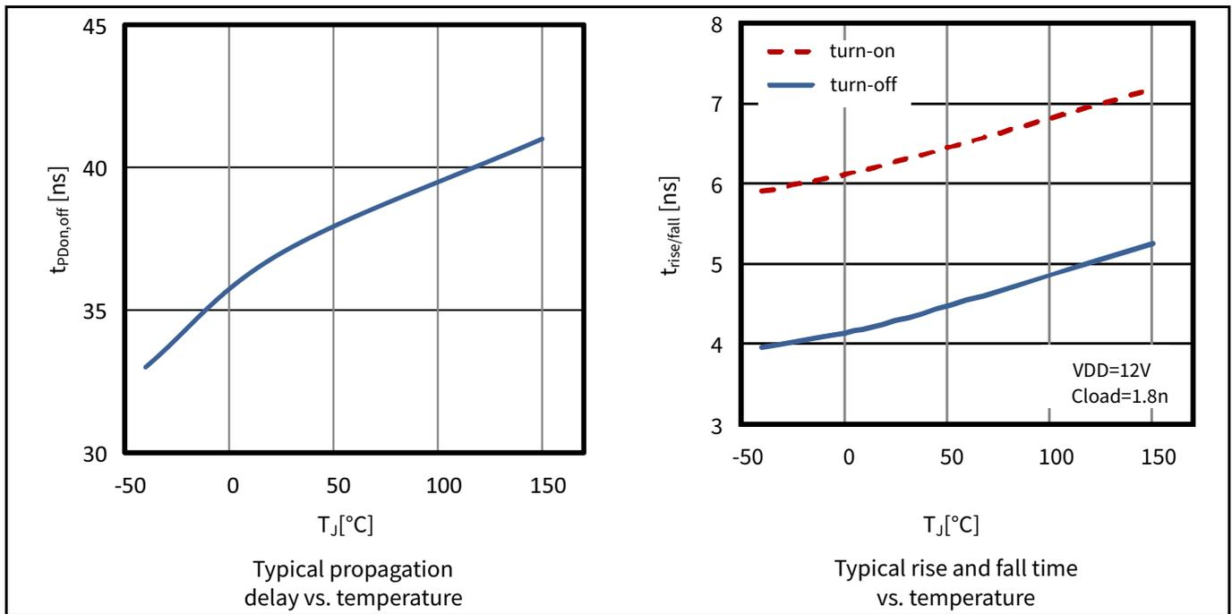
Figure 13 Propagation delay and rise / fall time
