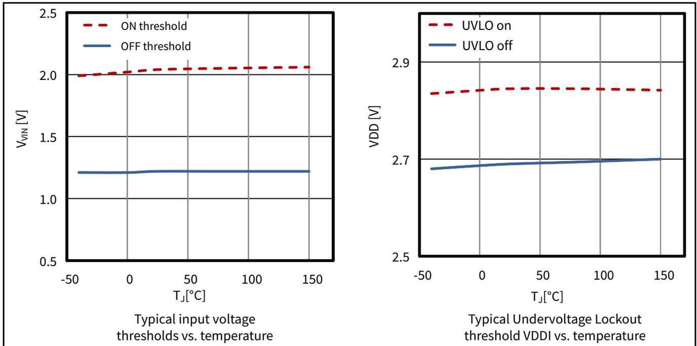
Figure 10 Logic input thresholds and VDDI UVLO
