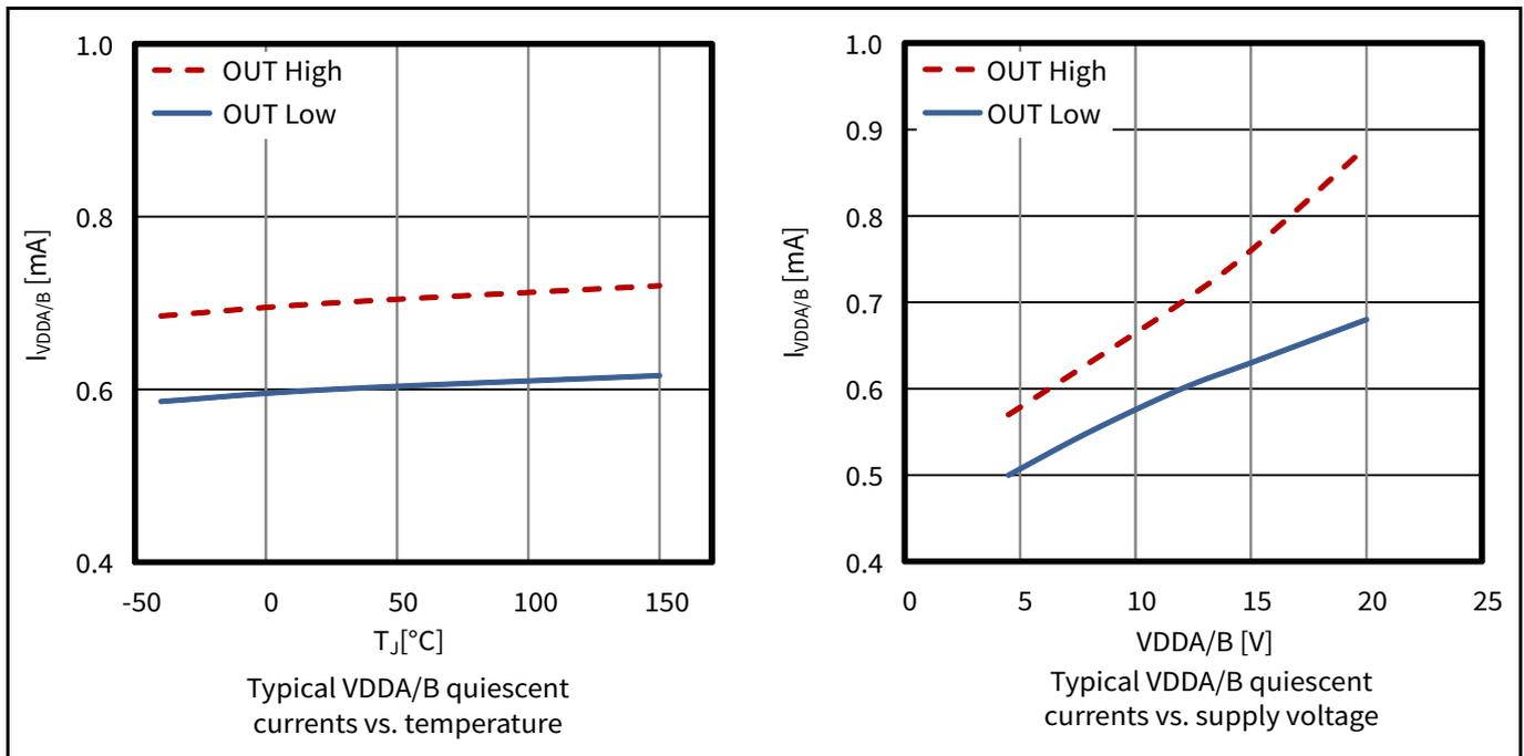
**Figure 7 Supply current VDDA, VDDB**
