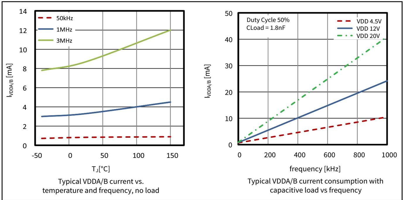
**Figure 8 Supply current VDDA, VDDB (with / without load)**
