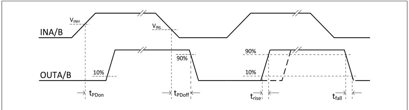
**Figure 4 Propagation delays, rise, fall and dead time**
