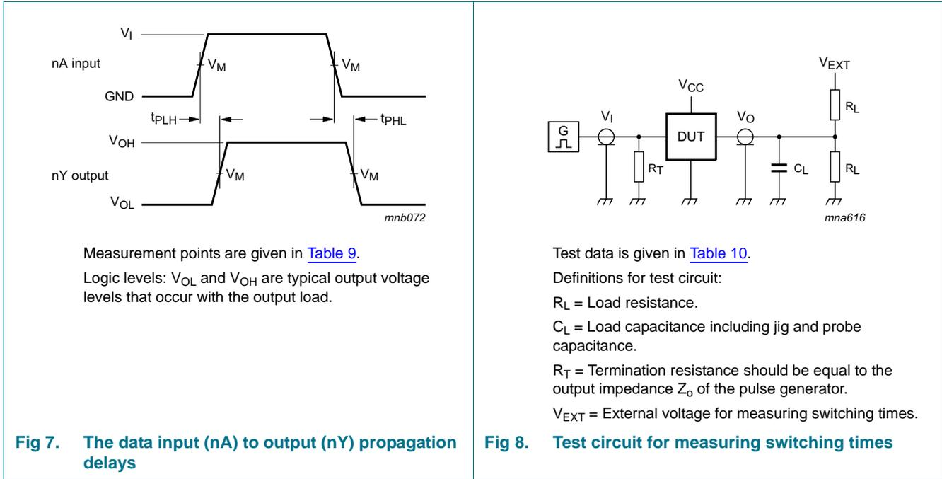
Fig 7. The data input (nA) to output (nY) propagation delays
