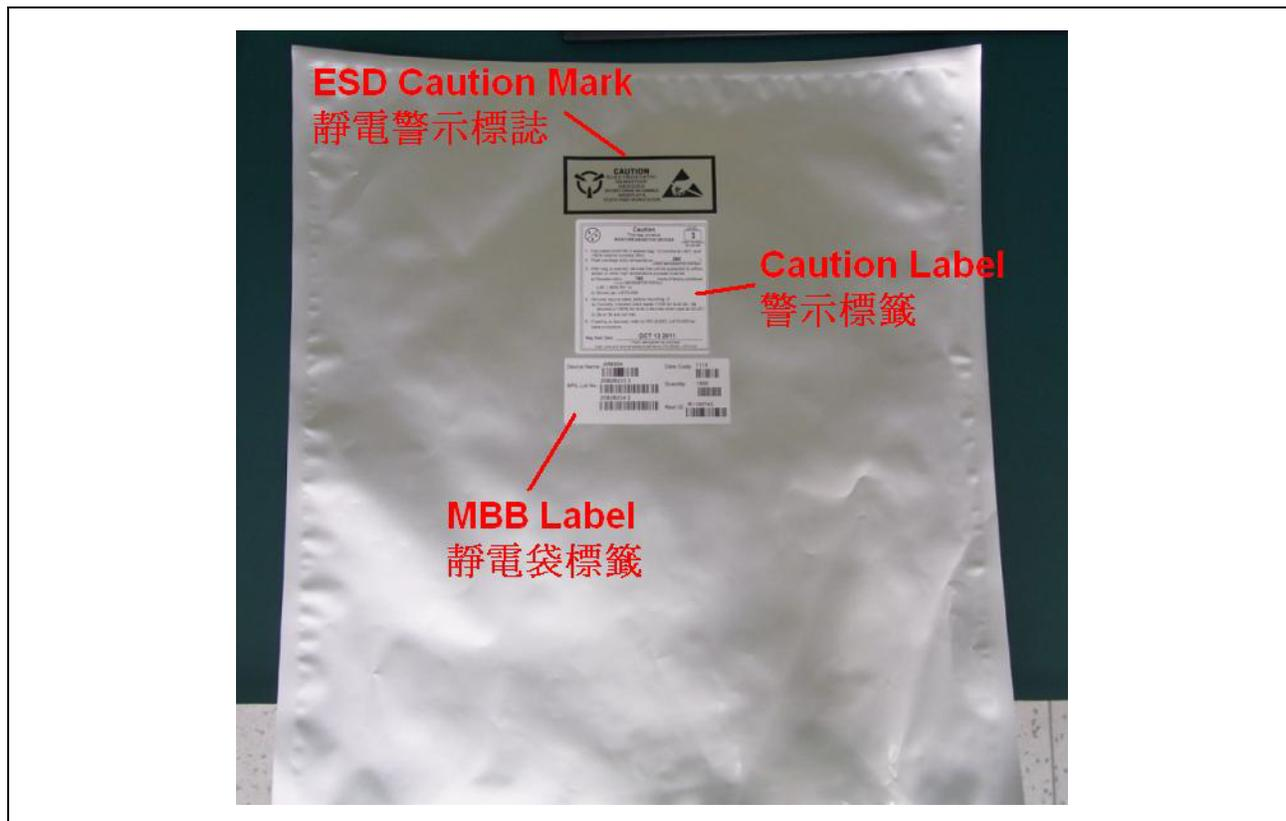
The moisture sensitivity label on the BCM20736S shipping bag is shown in [Figure 12 on page 25](#).
