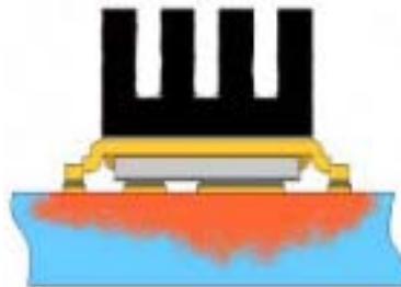
⑧ Mounted to a PCB with small clip heatsink (still air)
