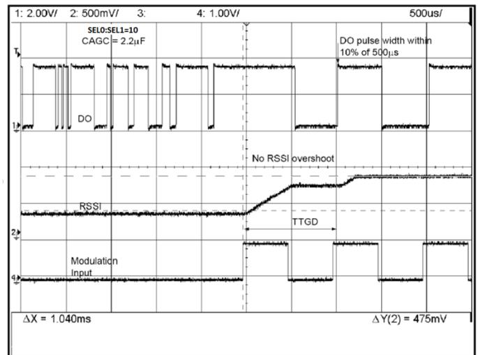
**Figure 5. Proper TTGD (1ms) with Sufficient AGC**
