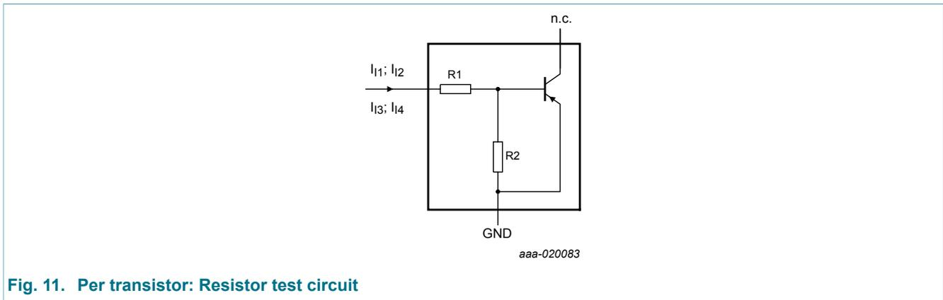
Fig. 11. Per transistor: Resistor test circuit
