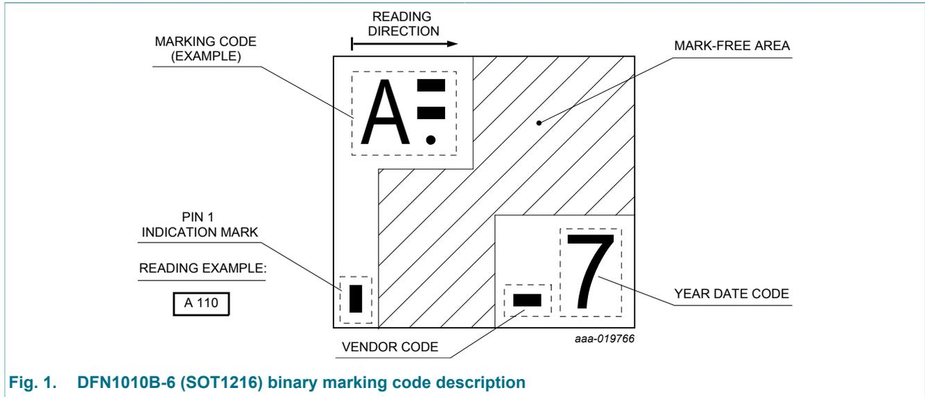
Fig. 1. DFN1010B-6 (SOT1216) binary marking code description
