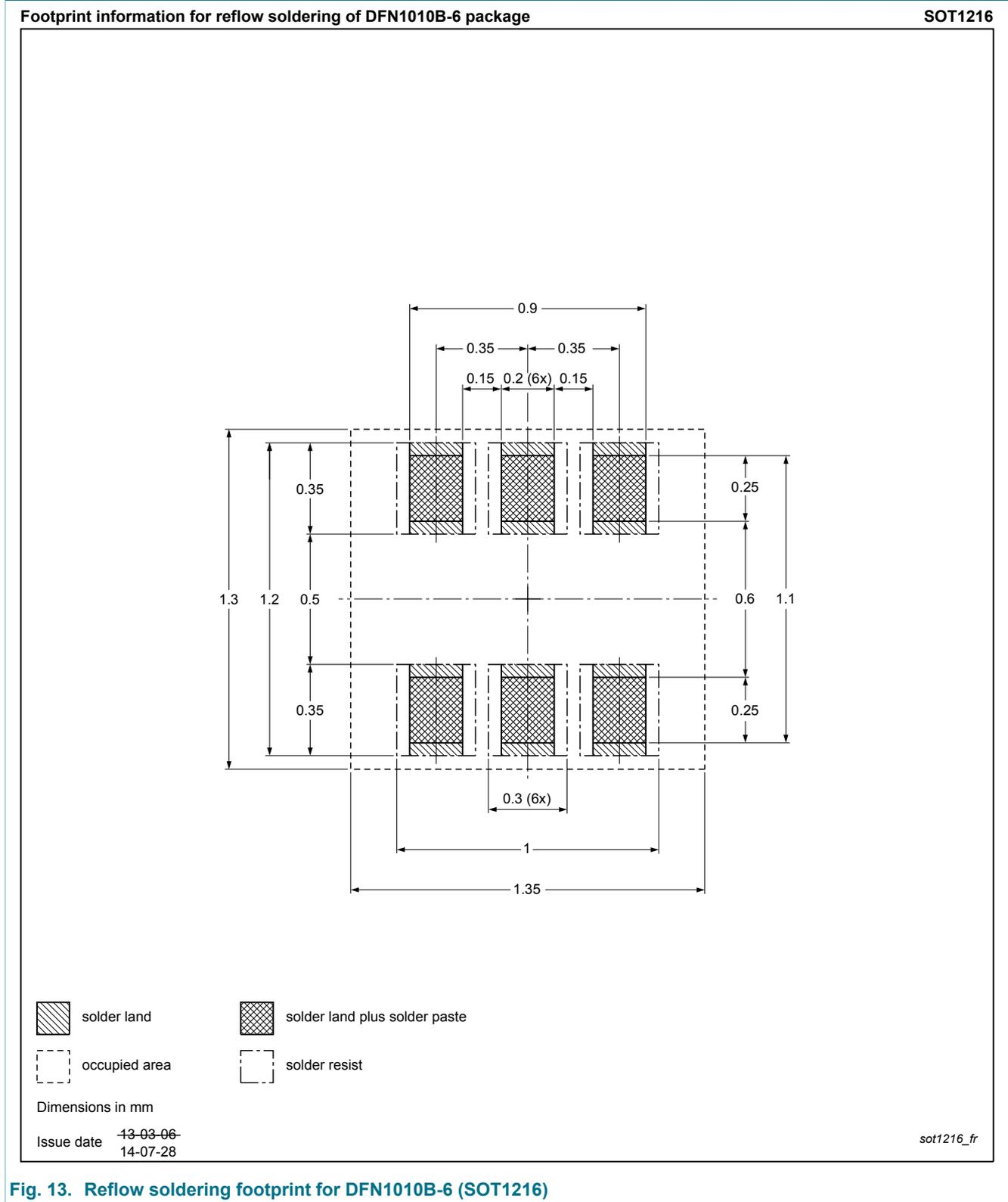
Fig. 13. Reflow soldering footprint for DFN1010B-6 (SOT1216)
