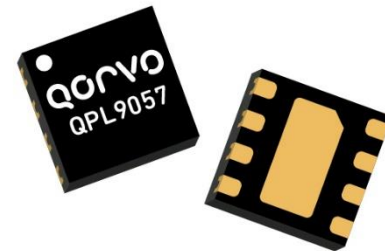
8 Pin 2X2 mm DFN Package
