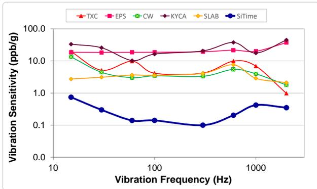
Figure 5. Vibration Robustness<sup>[5]</sup>
