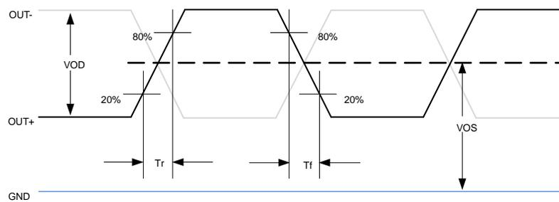
**Figure 2. LVDS Voltage Levels per Differential Pin (OUT+/OUT-)**
