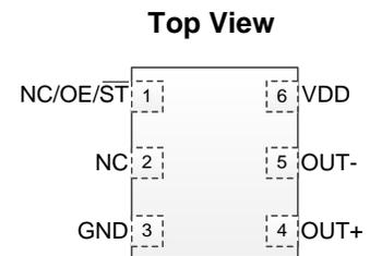
**Figure 1. Pin Assignments**
