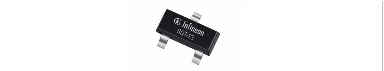
Figure 1 TLE4963-2M in the PG-SOT23-3-15 package
