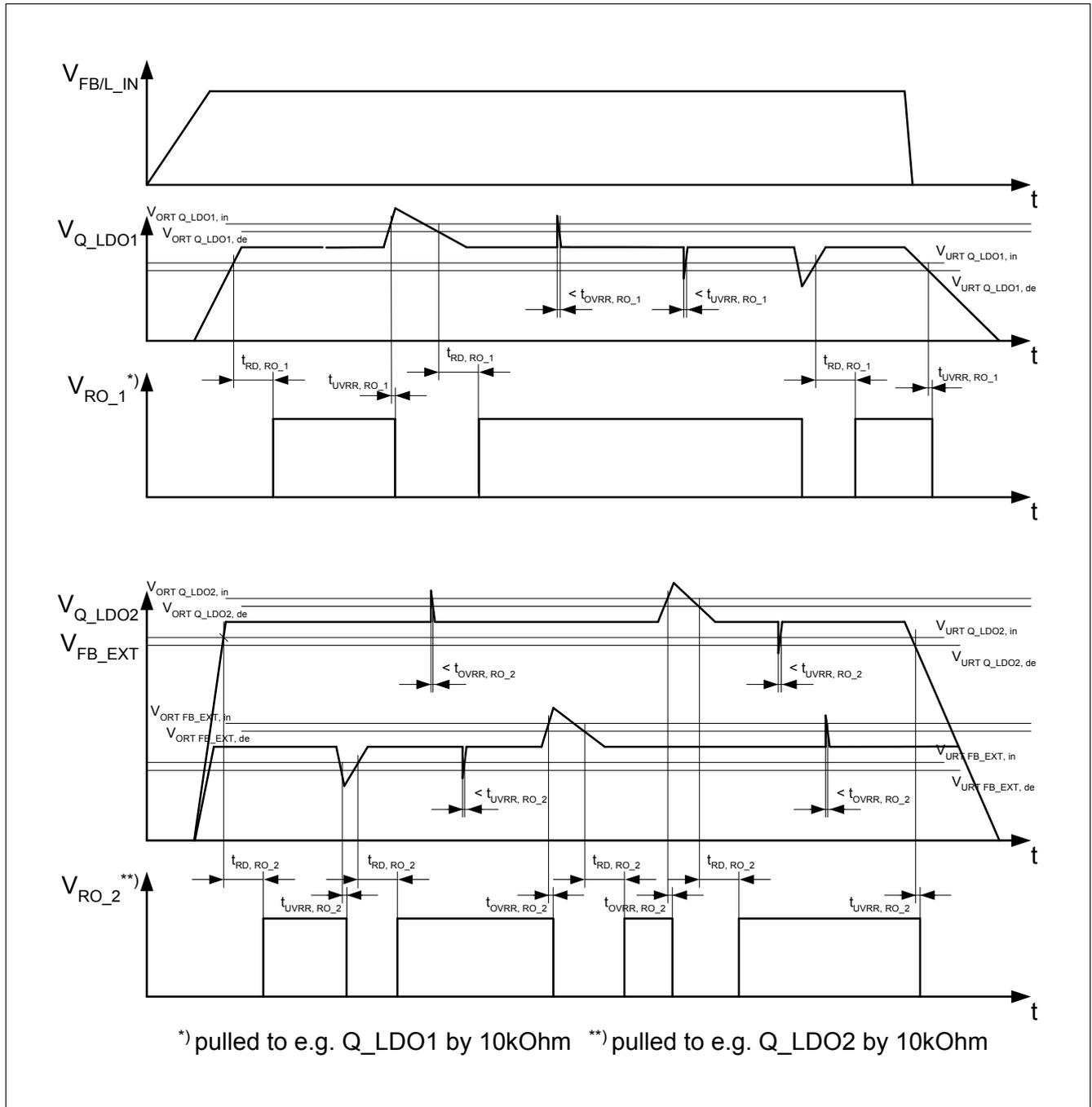
**Figure 5    Reset Timing TLE7368**
