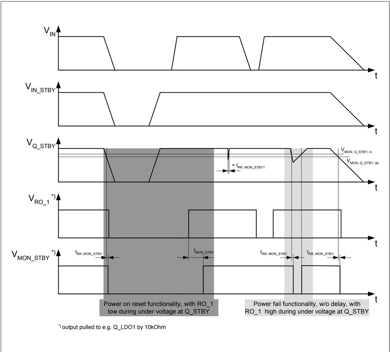
**Figure 7 Stand by Monitor Timing Diagram**
