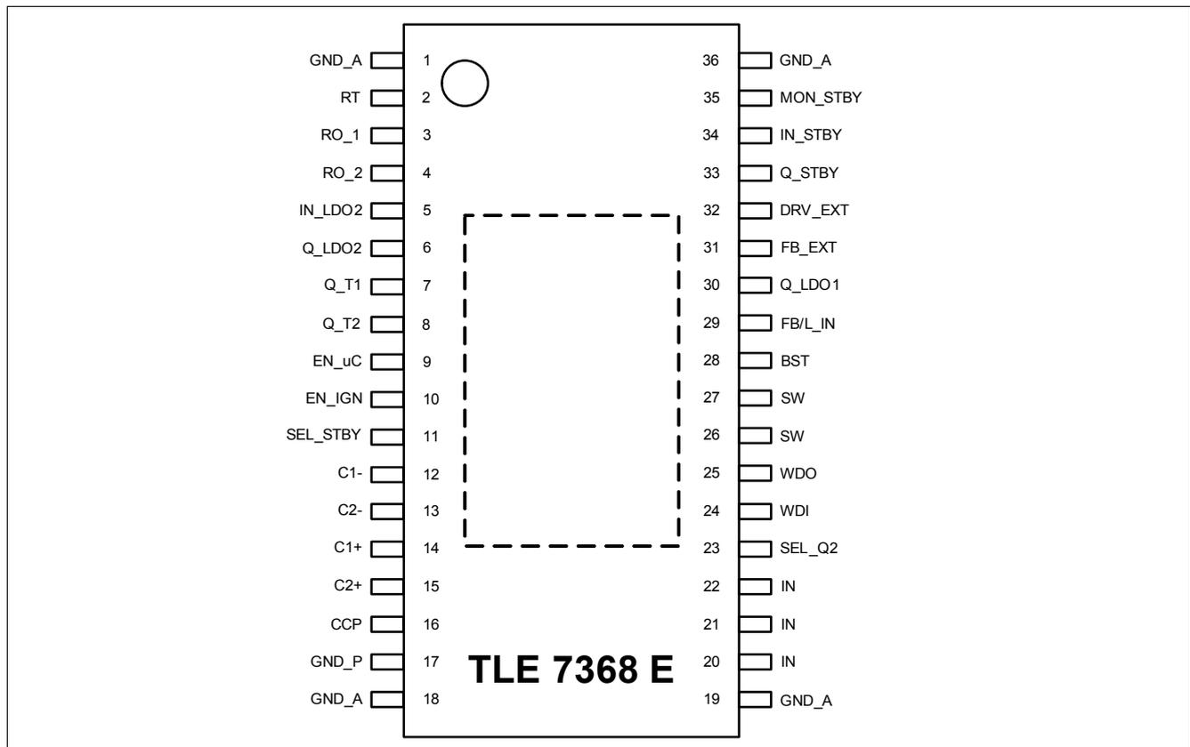
**Figure 2 Pin Configuration**
