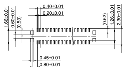
Recommended metal mask pattern Metal mask thickness: When 120μm (Terminal opening ratio: 70%) (Metal-part opening ratio: 100%)
