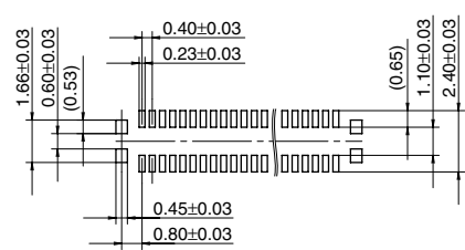
Recommended metal mask pattern Metal mask thickness: When 120μm (Terminal opening ratio: 70%) (Metal-part opening ratio: 100%)
