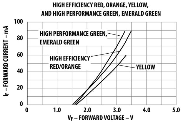
Figure 2. Forward current vs. forward voltage (non-resistor lamp).
