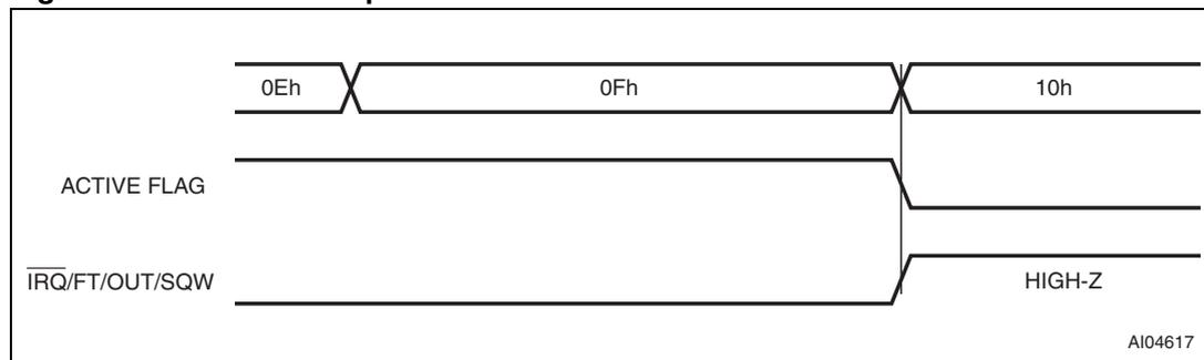
Figure 13. Backup mode alarm waveform
