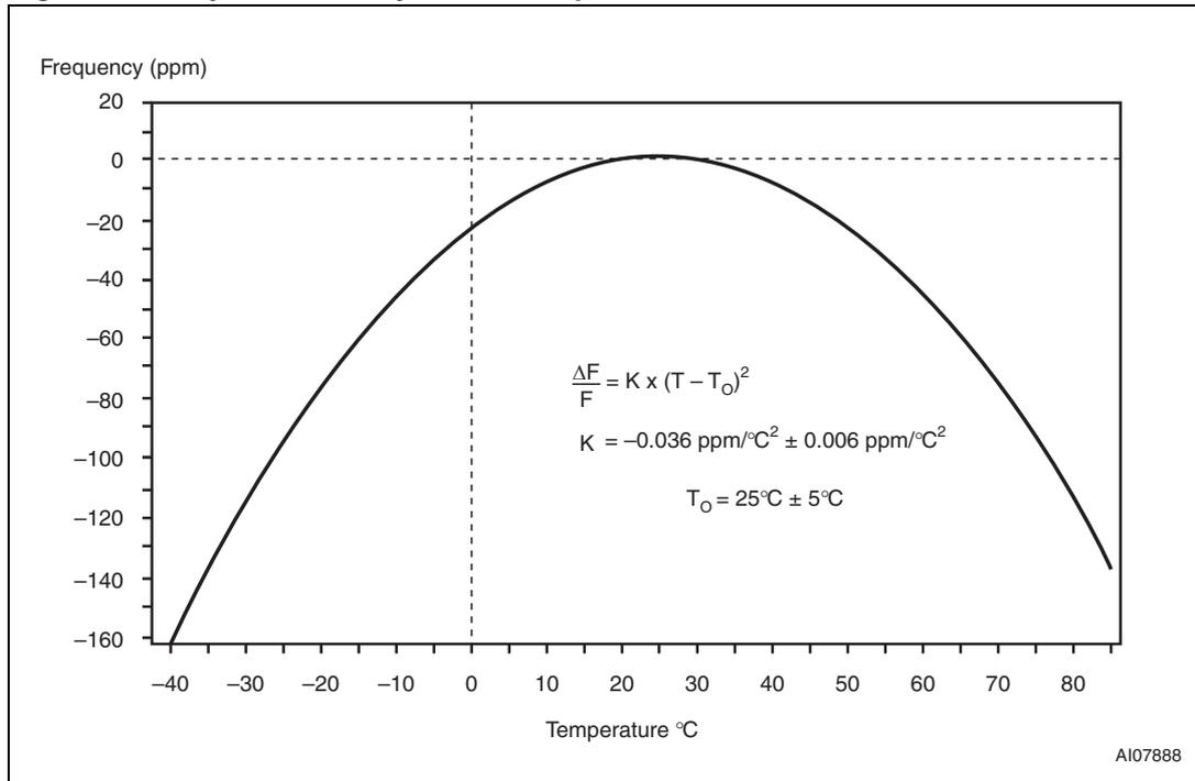
**Figure 11. Clock calibration**
