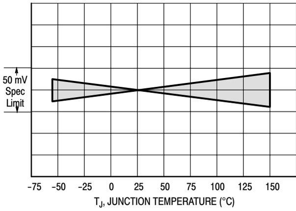
Figure 2. Reference Stability over Temperature
