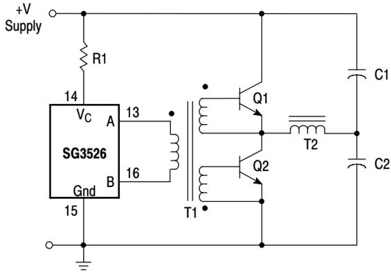
Figure 19. Half-Bridge Configuration
