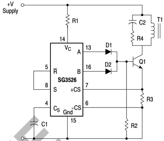
In the above circuit, current limiting is accomplished by using the current limit comparator output to reset the soft-start capacitor.
