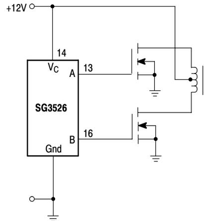
The totem pole output drivers of the SG3526 are ideally suited for driving the input capacitance of power FETs at high speeds.
