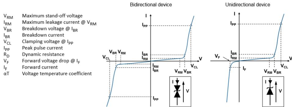
**Figure 2. Pulse definition for electrical characteristics**
