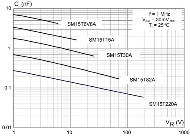
**Figure 8. Junction capacitance versus applied voltage (bidirectional type)**
