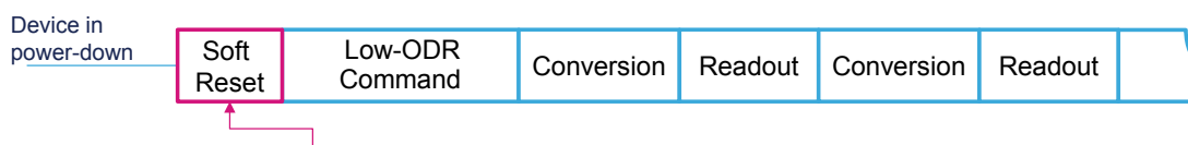
Figure 8. Low-ODR mode enable sequence
