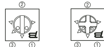
3314J-3, G-3, R-3, H-3 (Reverse Marking, Straight Slot) 3314J-4, G-4, R-4, H-4 (Reverse Marking, Cross Slot)
