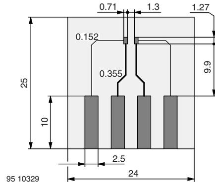
Figure 4. Board for  $R_{thJA}$  Definition (in mm)
