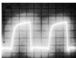
Signal Waveform (20ns/div, 1V/div)
