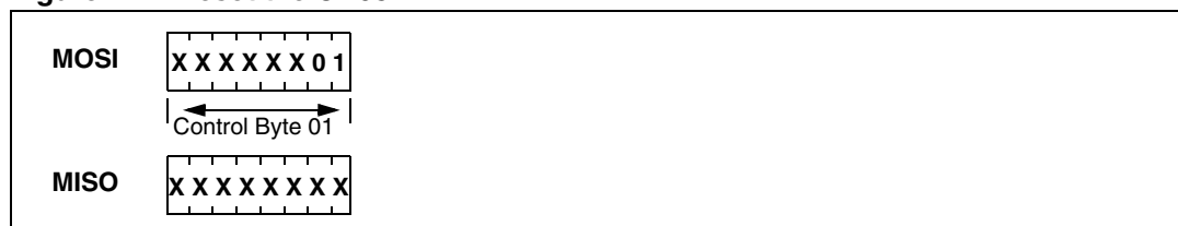
Figure 11. Reset the CR95HF
