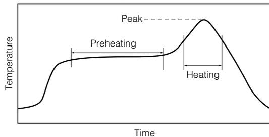
For soldering (Example : Sn/Pb)
