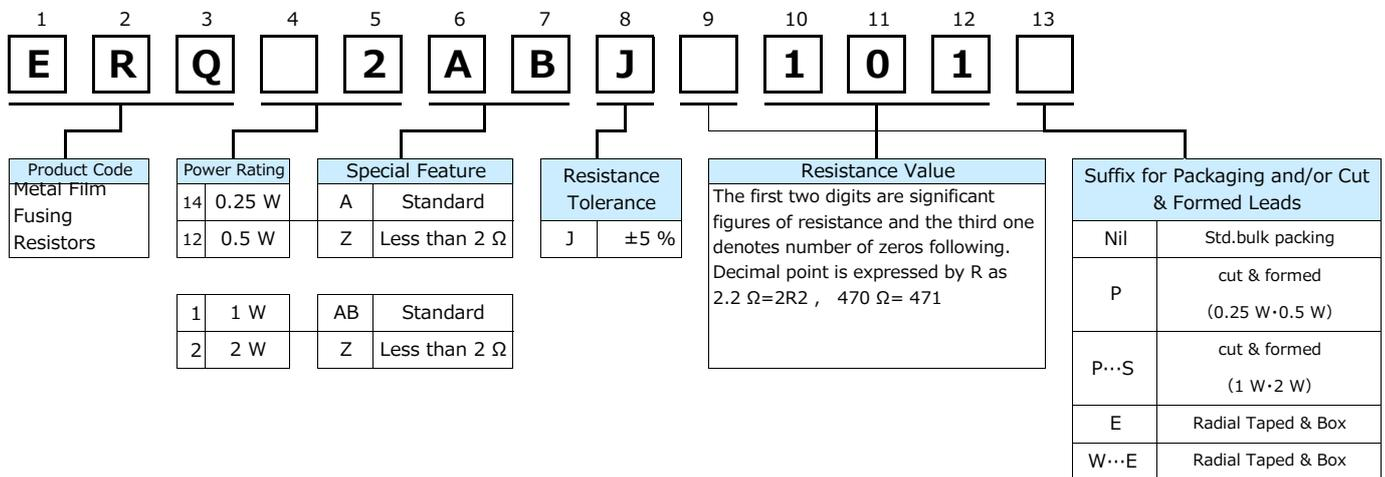
The above example shows a standard Metal Film Fusing Resistors, 2 W power rating, resistance value of 100 Ω, tolerance of ±5 %, and package of standard bulk packing.
