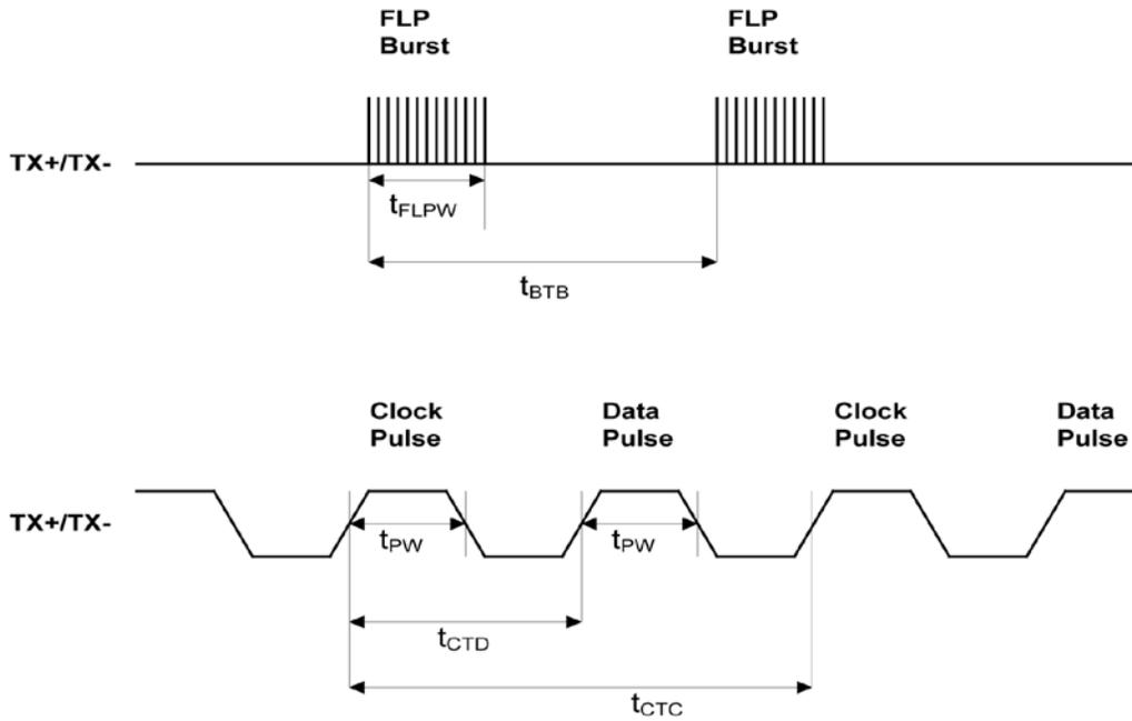
Figure 16. Auto-Negotiation Fast Link Pulse (FLP) Timing
