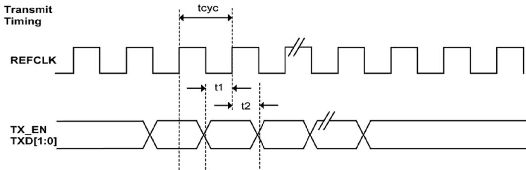
**Figure 14. RMII Timing – Data Received from RMII**
