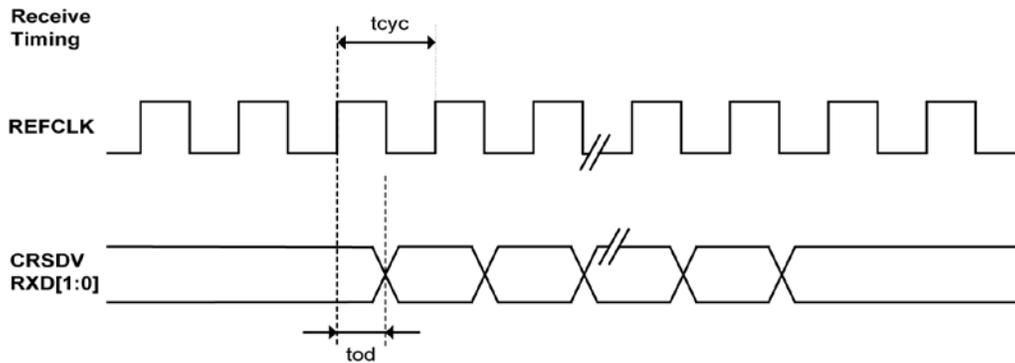
**Figure 15. RMII Timing – Data Input to RMII**
