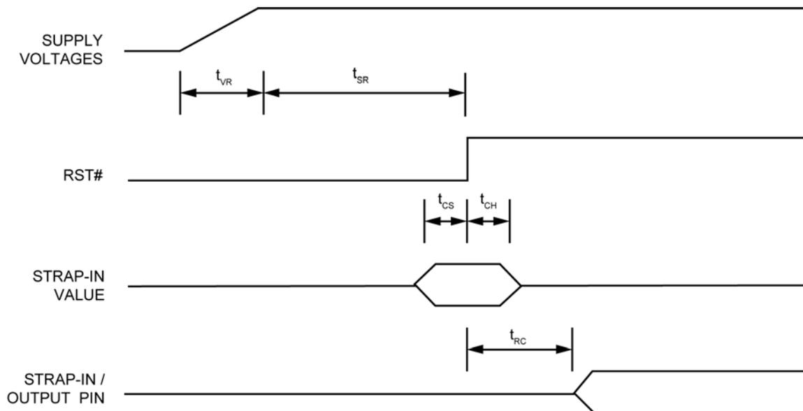
Figure 18. Power-Up/Reset Timing
