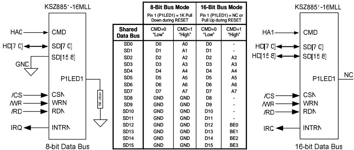
Figure 6. KSZ8851-16MLL 8-Bit and 16-Bit Data Bus Connections
