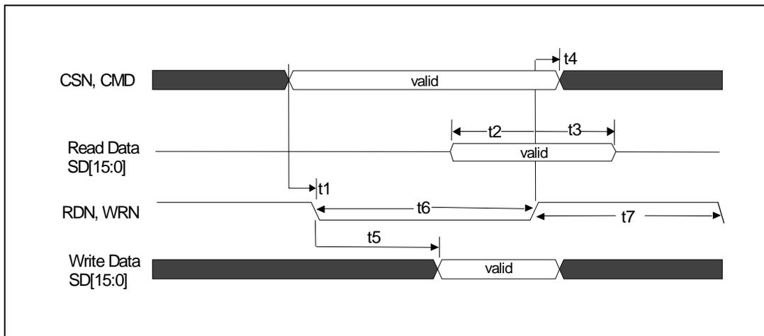
Figure 11. Asynchronous Cycle
