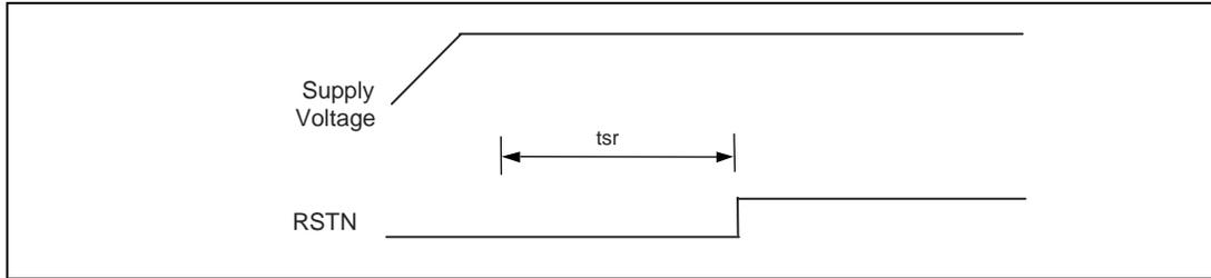
**Figure 13. Reset Timing**
