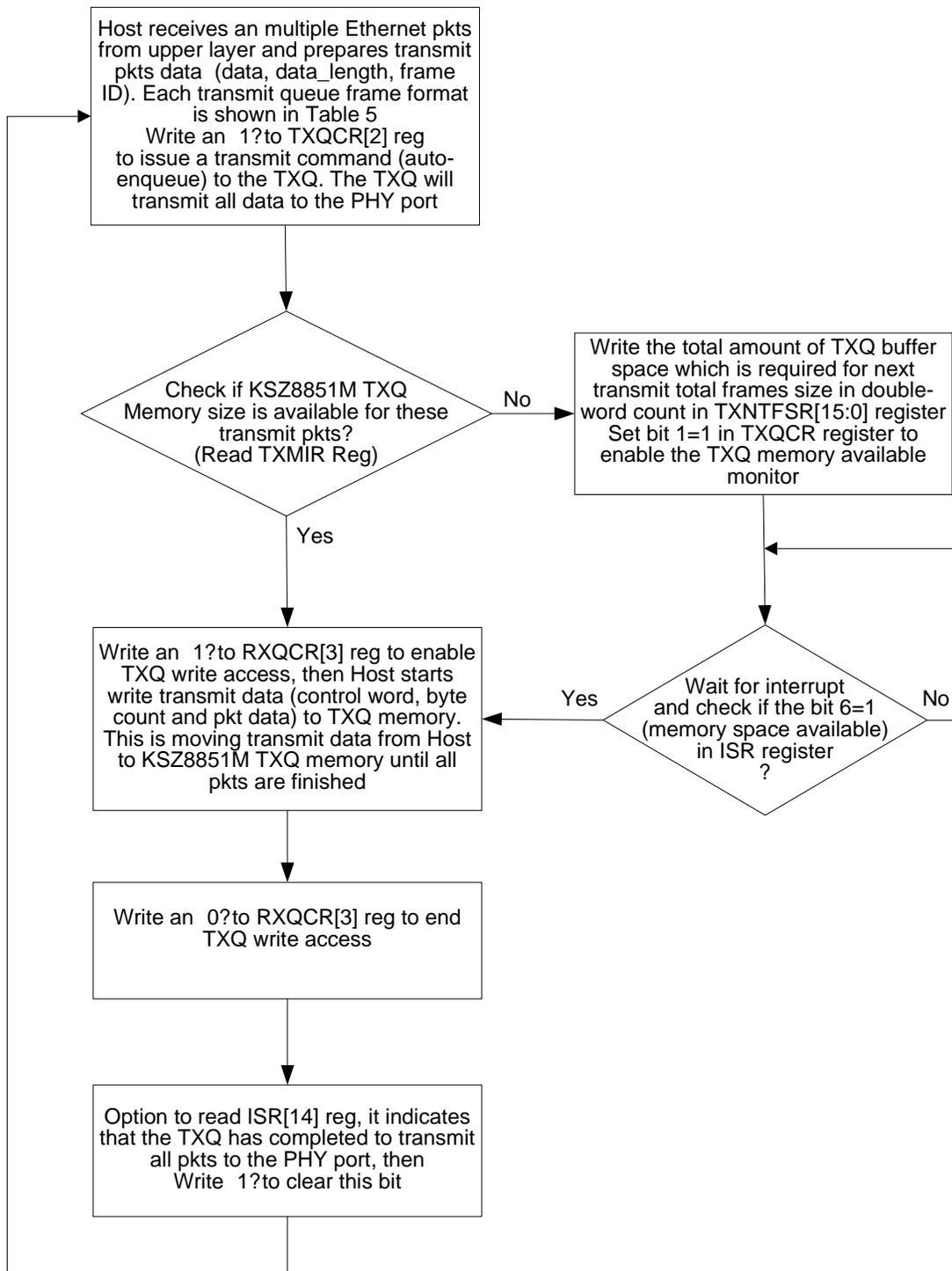
Figure 8. Host TX Multiple Frames in Auto- Enqueue Flow Diagram
