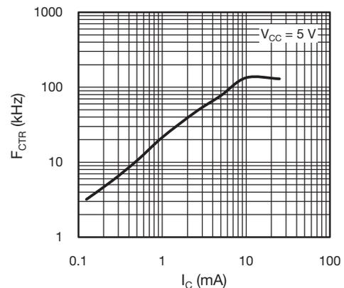
Fig. 12 - F<sub>CTR</sub> vs. Collector Current
