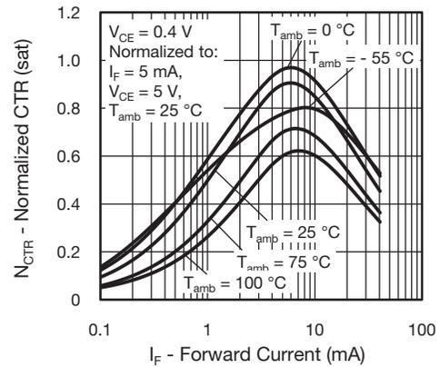
Fig. 10 - Normalized CTR (sat) vs. Forward Current
