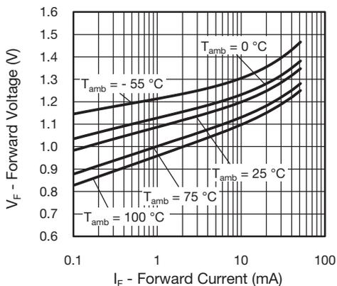
Fig. 3 - Forward Voltage vs. Forward Current
