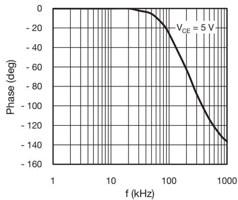
Fig. 11 - F<sub>CTR</sub> vs. Phase Angle
