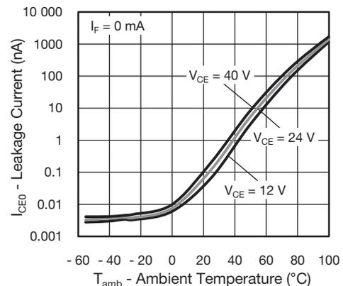
Fig. 5 - Leakage Current vs. Ambient Temperature
