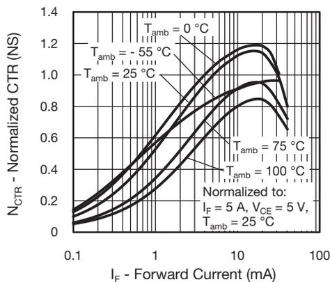
Fig. 9 - Normalized CTR (NS) vs. Forward Current
