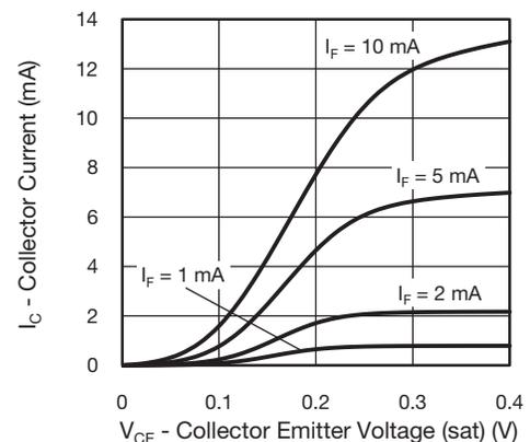
Fig. 6 - Collector Current vs. Collector Emitter Voltage (sat)
