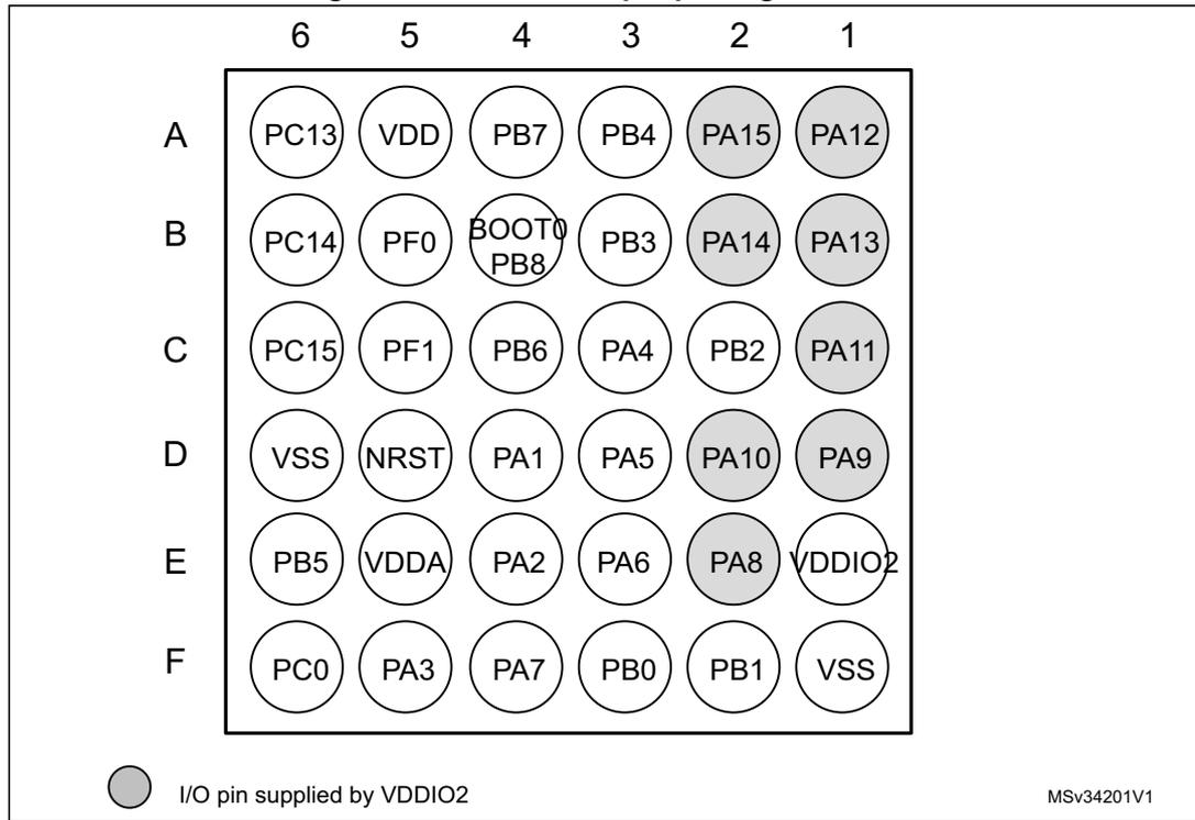
Figure 6. LQFP32 32-pin package pinout (top view)
