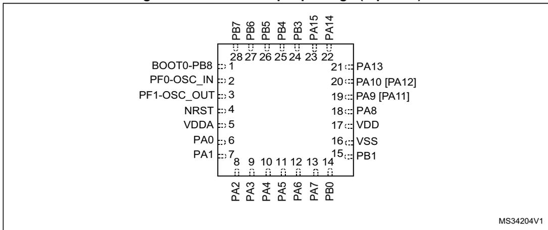
1. Pin pair PA11/12 can be remapped instead of pin pair PA9/10 using the SYS\_CTRL register.
