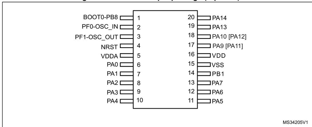
1. Pin pair PA11/12 can be remapped instead of pin pair PA9/10 using the SYS\_CTRL register.
