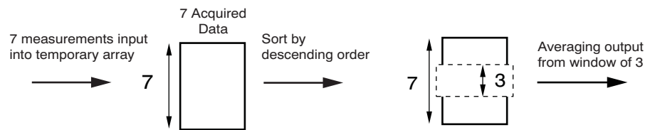
Figure 28. MAV Filter Operation
