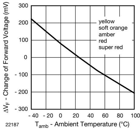
Figure 7. Change of Forward Voltage vs. Ambient Temperature
