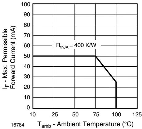
Figure 1. Max. Permissible Forward Current vs. Ambient Temperature
