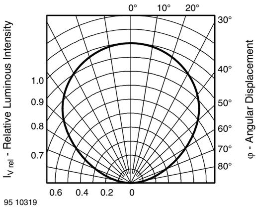
Figure 2. Rel. Luminous Intensity vs. Angular Displacement
