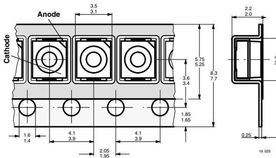
Figure 10. Tape Dimensions in mm for PLCC-2
