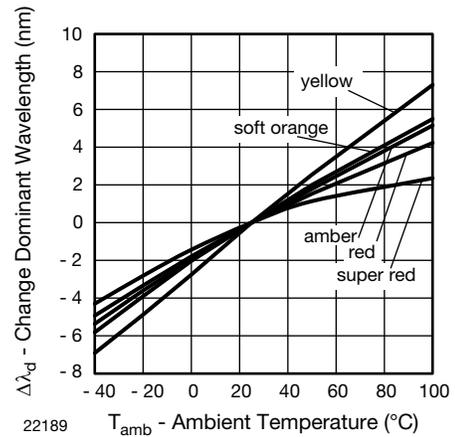
Figure 9. Change of Dominant Wavelength vs. Ambient Temperature
