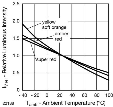
Figure 8. Relative Luminous Intensity vs. Amb. Temperature
