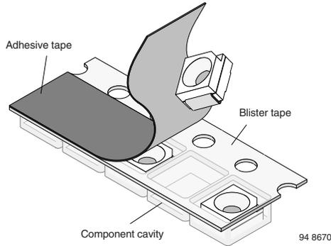
REEL PACKAGE DIMENSION IN MILLIMETERS FOR SMD LEDS, TAPE OPTION GS08 (= 1500 PCS.)
