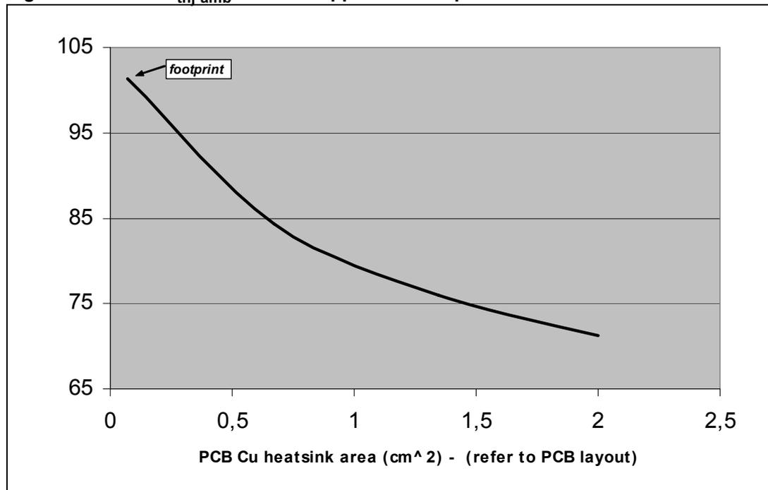
Figure 36. SO-8 thermal impedance junction ambient single pulse
