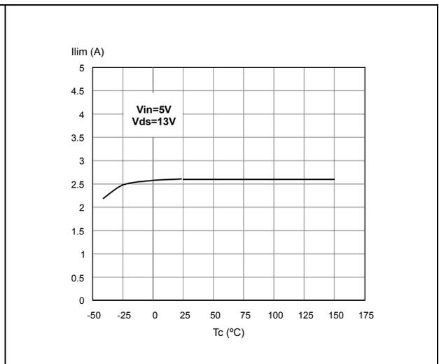
**Figure 29. Step response current limit**
