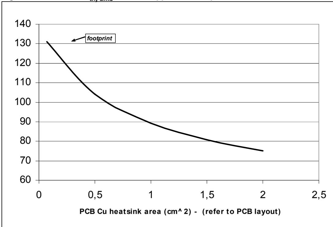
Figure 32. SOT-223 thermal impedance junction ambient single pulse
