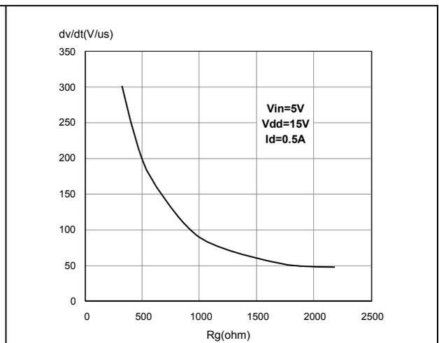
**Figure 21. Turn-off drain-source voltage slope (part 2/2)**      **Figure 22. Capacitance variations**
