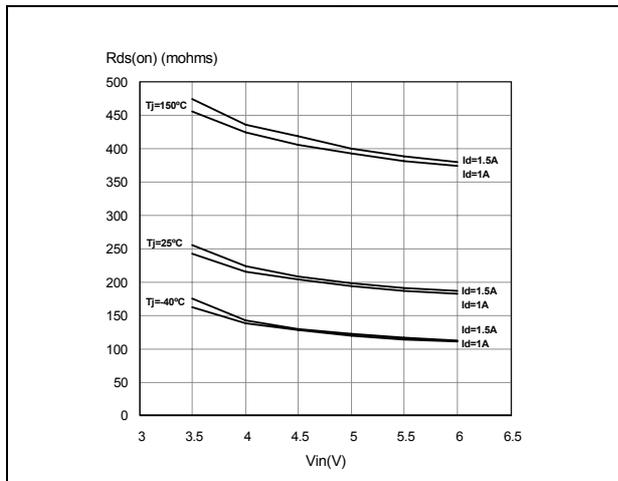
**Figure 10. Static drain-source on resistance**
