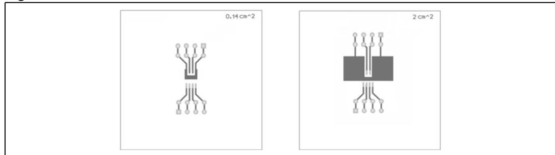
Note: Layout condition of  $R_{th}$  and  $Z_{th}$  measurements (PCB FR4 area = 58 mm x 58 mm, PCB thickness = 2 mm, Cu thickness = 35 μm, Copper areas: from minimum pad layout to 2 cm<sup>2</sup>).
